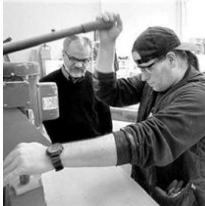
CREDIT: Darren Stone, Times Colonist Assistant cabinet maker Joe Ladouceur uses a multi-drill machine with Renaissance Cabinets owner Azim Virjee.
